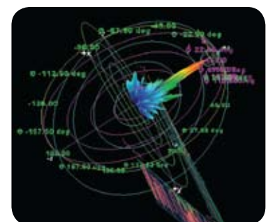
3D image of antenna far field radiation pattern
