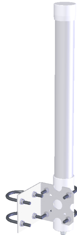
MOUNTS TO Ø 57 OMNI ANTENNAS VIA M8 U-BOLTS (MK4/C)
