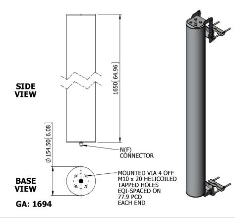
ELECTRICAL Frequency 960-1220 GHz Gain 13 dBi Typ Polarisation Linear (Vertical) Beamwidth 110° (Az) x 9° (El) Approx Cross Polar >20 dB Typ VSWR 2:1 Max 100 W Power Rating Front to Back >20 dB MECHANICAL Standard Finish Camouflage Grey Mass 5.7 Kg excl Mounting Kit Temperature - Operating -33°C to 55°C Temperature - Storage -55°C to 71°C Wind Loading 41.4 Kg (90 lbs) @ 100 mph MOUNTING OPTIONS Kits Available 051A Supplied See separate data sheets ADDITIONAL NOTES
