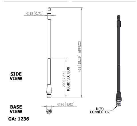
Gain 2 dBi Nom Polarisation Linear (vertical) Beamwidth 360° (Az) x 80° (El) Cross Polar 25 dB Typical VSWR 2:1 25W Power Rating Front to Back N/A MECHANICAL Standard Finish Matt Black Mass 180g (0.39 lbs) approx Temperature -20° to +50°C Wind Loading N/A MOUNTING OPTIONS
