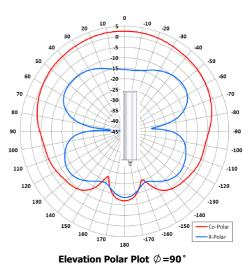
**ELECTRICAL** Frequency: 400 - 408 MHz Gain: 3 dBiC Nom. **Polarisation:** Left Hand Circular 360° (Az) x 160° (El) Beamwidth: **Axial Ratio:** 3 dB Typ. **VSWR:** 2:1 Max. **Power Rating:** 50 W
