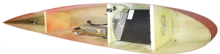
Inside the wing-tip of the experimental aircraft G-SMLI modified for survey work and wildlife tracking, showing the CAS antenna, with electrical tilt-ability.
