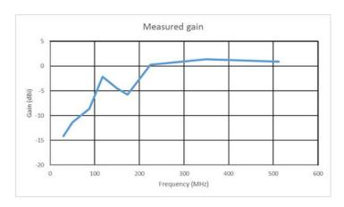
Gain figures for the antenna apply when mounted on a 2.4m diameter nominal conductive flat groundplane.
