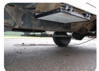
High power planar spiral antenna mounted under vehicle provide countermeasures
